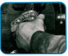
Lock the pinion shaft in the vice again. Apply threadlocker to a new pinion nut, then tighten it until bearing end play is removed. Wrap a rope around the pinion housing and attach a fish scale to the free end. Correctly adjusted new bearings require a 10-15 pound pull to rotate the housing.
