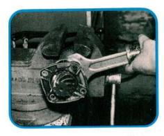
Use a 47 mm wrench or a really large crescent wrench to loosen the pinion bearing retaining nut. The Saab tool number for their wrench is 87 90 453. Notice the added persuasion at the end of the wrench. The nut was peened over and had threadlocker on it to boot. Never reuse the nut.
