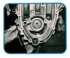
Reinstall fifth gear and its selector assembly. Slide the shift fork over the selector shaft, then reinstall its locating pin. Hold the selector collar and fork in this position while guiding the transfer gear and bearing into the front of the primary gear case.
