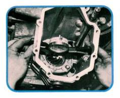
The correct pinion depth setting for each ring and pinion set is scribed on the pinion. This pinion was marked -5, meaning -.05 mm. There's a pinion depth tolerance of  $\pm.05$  mm. The Saab dial indicator must be used to measure the pinion depth when a new housing is installed.
