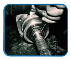
After a few tries, you may be able to tell how 10-15 pounds feels by rotating the housing by hand. Don't take chances until you do. Never loosen the pinion nut if it's overtightened. Replace the crush sleeve and start over. After properly torquing the nut, peen it with a punch.
