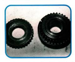
Fourth gear (right) should spin freely on the pinion shaft. A broken pinion housing will push fourth gear against the 3-4 synchronizer hub (left). The added friction and heat can weld the synchronizer hub and gear together, leaving you stranded in fourth gear.
