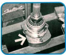
This press plate (arrow) prevents damage to the pinion gear when removing the pinion bearings and housing. Different plates are used for different final drive ratios. Use 87 91 097 for 1982 and later 900s. The plate removes both bearings and the housing from the
