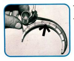
Check the shift forks over carefully. If the owner is in the habit of driving with his hand resting on the shift lever, the fork may wear in this area (arrow) from rubbing against the shift collar. Match each fork to its shift rod and check for excessive wear between the two.
