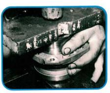
Use an old outer bearing race as a drift to install both new bearing races. The edge of the housing is chamfered so the old race can't get stuck in the housing. The races bottom against recessed shoulders. Don't apply 20 tons trying to close the shoulder gap. It's supposed to be there.
