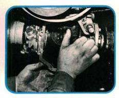
If you don't have a measuring instrument built into your wrist, check backlash with a dial indicator. The specification is 0.17 mm  $\pm$ .05 mm. Mount the indicator button perpendicular to the ring gear tooth. Reinstall the differential cover, then refill the transmission.
