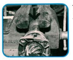
Necessity is the mother of invention, and I'm not talking about Frank Zappa. A scrap synchronizer hub (arrow) does a good job of holding the pinion shaft in the vice. The factory tool does exactly the same thing. Use one or the other, but never clamp the pinion shaft directly in the vice.
